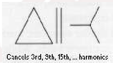
ISOLATION (DELTA-STAR) (ARRESTS ALL TRIPLEN )
